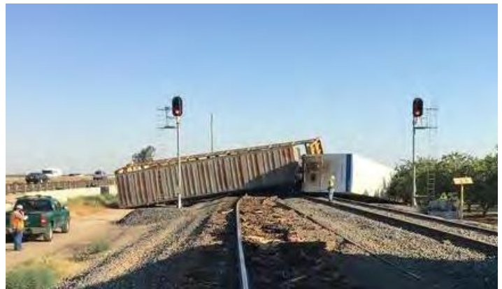
Derailment from railway buckling occurred in Tulare County in 2017
